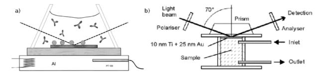
Imaging ellipsometry has been reported to allow measuring more than 105 pixels on an area of less than one  $cm^2$  in one second. For this technique a CCD camera was used as a detector. ELM allows determining the thickness of solid thin-films in air with accuracy well below 1 Angstrom, the detection limit for the adsorption of biomolecules is average: A detection limit of around 1 ng/cm<sup>2</sup> has been reported for surface plasmon enhanced ellipsometry [81].
